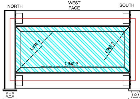
**Figure 7 Lines of Local Buckling Specimen C1**
