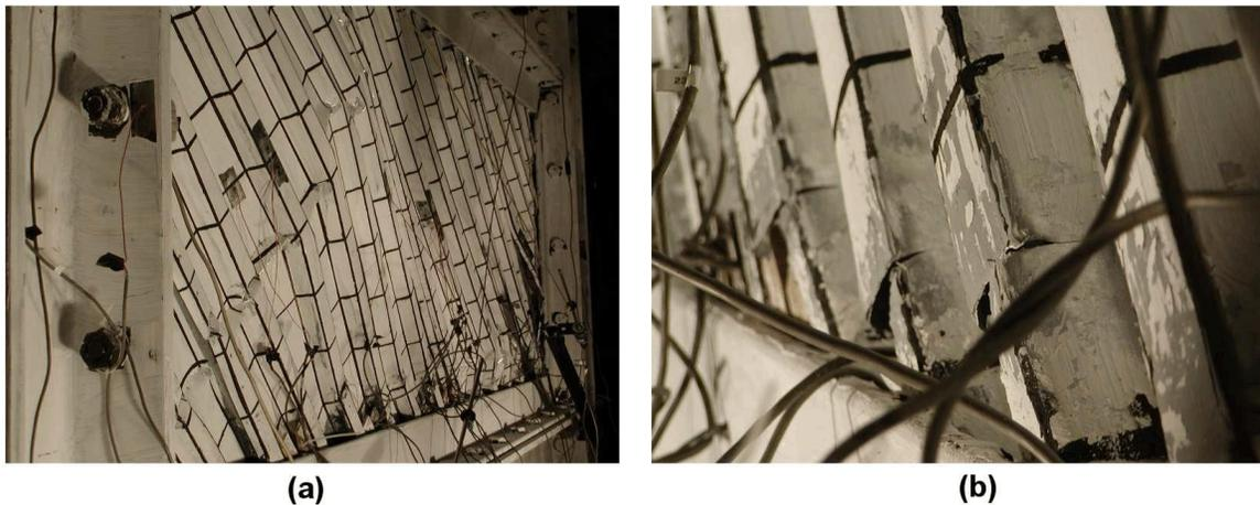
**Figure 8 Specimen C1; (a) Buckling of Infill (b) Fracture Along Line 2**
