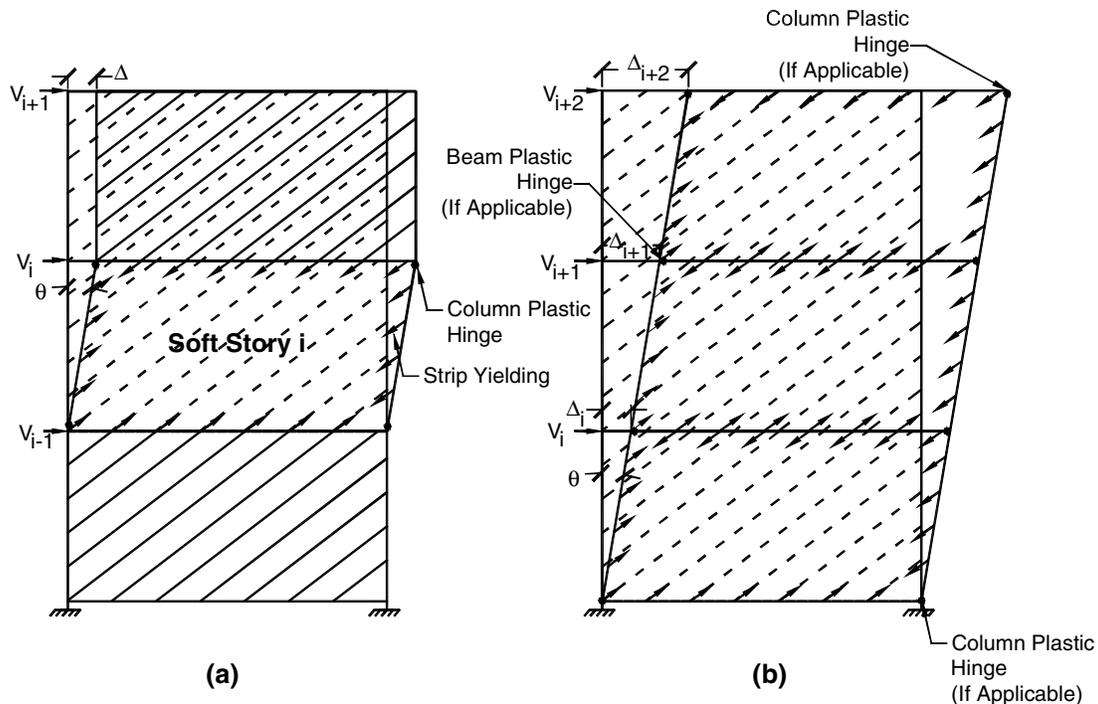
**Figure 3 (a) Soft-Story Collapse Mechanism (b) Uniform Yielding Mechanism**
