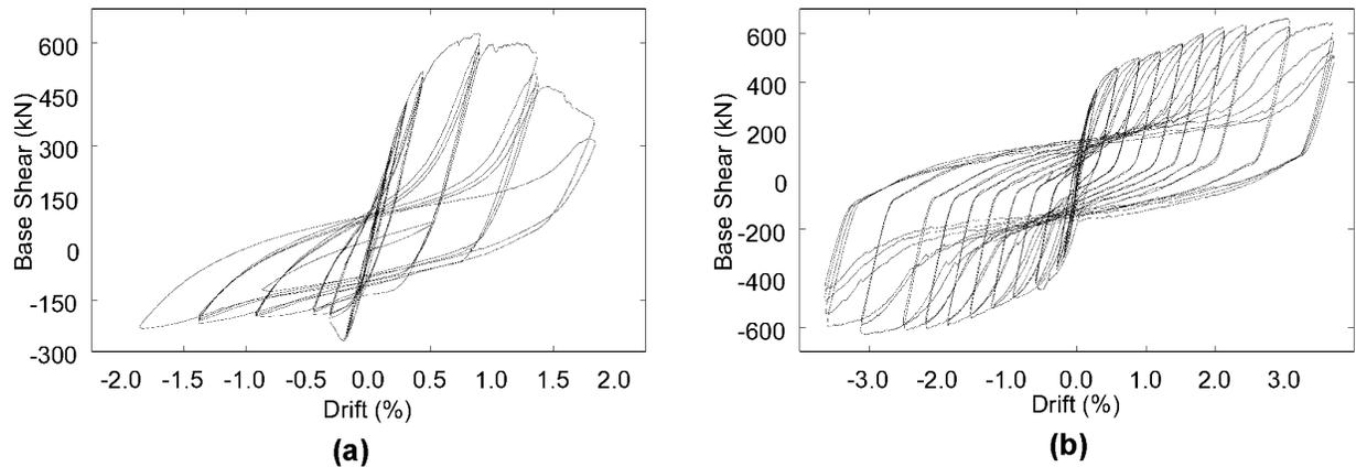
**Figure 9 Specimen Hystereses; (a) Specimen C1 (b) Specimen F2**
