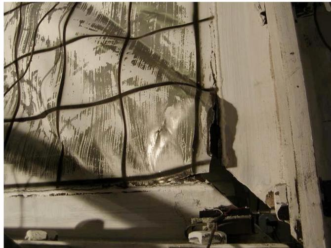
**Figure 10 Fracture of Infill - Specimen F2**
