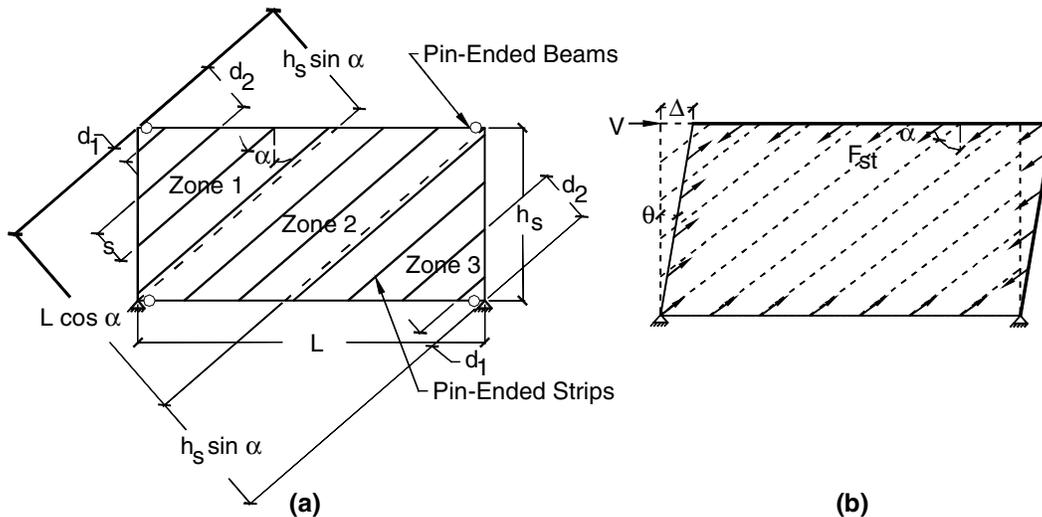
Figure 2 (a) Single Story Strip Model (b) Single Story Collapse Mechanism
